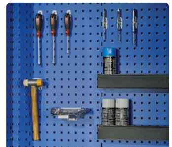
Perforated interior walls for systematic storage of tools and stored goods using perforated wall hooks and storage shelves.
